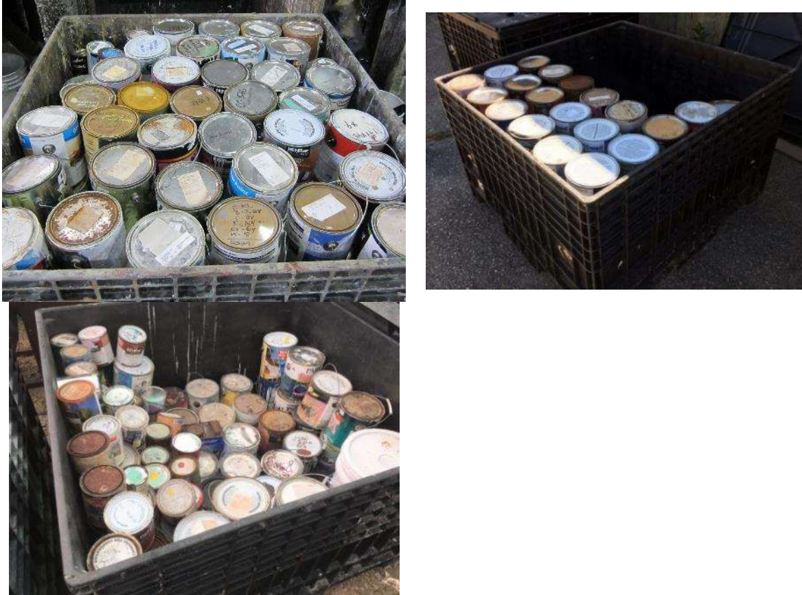
FIGURE 5: CORRECTLY PACKED TUBSKIDS
