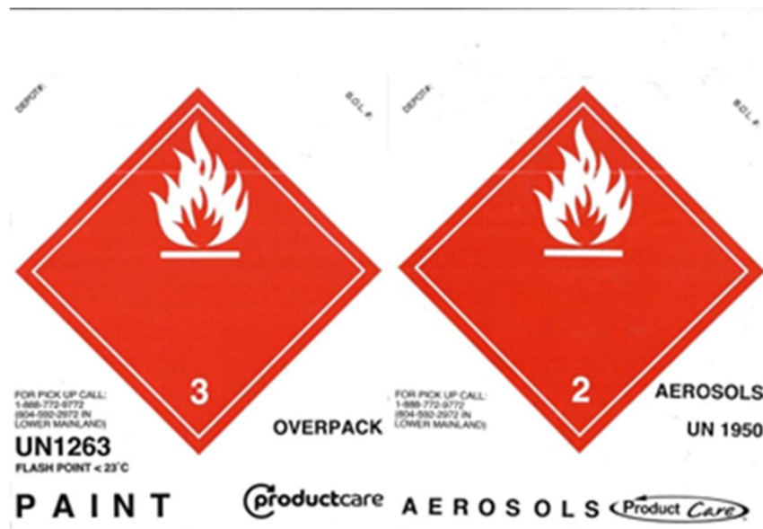
FIGURE 6: HAZARDOUS COLLECTION CONTAINER LABELS
